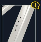
The **lower** position of the inserts is reserved for the **water bottle holder**, while the <u>upper</u> position is exclusive to the <u>Bosch powermore battery extention</u>.
