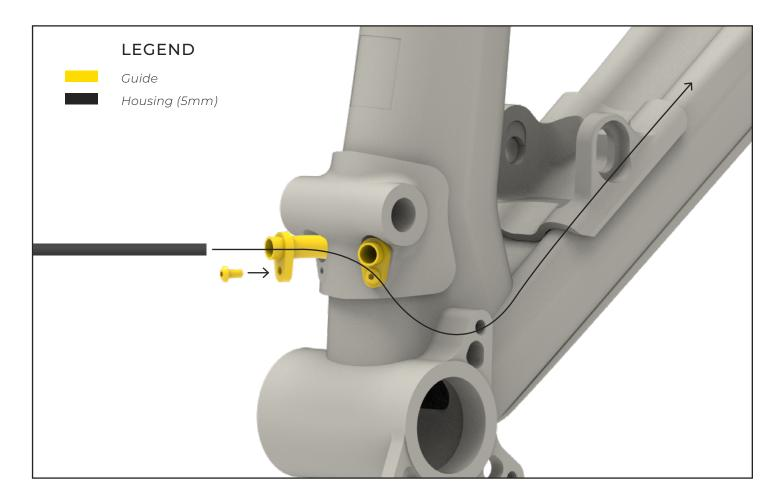
**STEP 1** | To orient the guide correctly through the downtube, take a 5mm housing and insert it into
