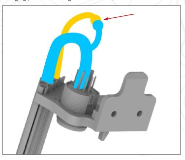
**Step 4.2** | Step 2.2 | Step 3.2 | Introduce the cables into the cable guide while making sure to nest the wires in their respective base. (See annex 1.1)
