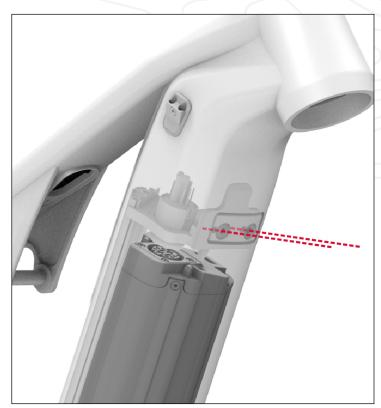
**Step 4.4** | Step 2.4 | Step 3.4 | Once the cable guide is fully inserted in the diagonal, ensure that it is correctly positioned by guiding you using the battery.
