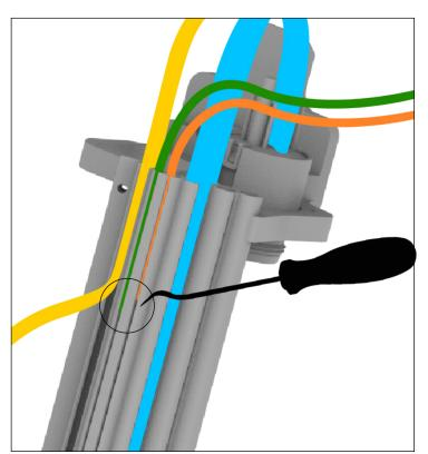
**Step 4.3** | Step 2.3 | Step 3.3 | Introduce slowly the cable guide inside the diagonal while nesting the motor support cable in its base. while sliding the cable guide in the diagonal, simultaneously help yourself with a hook to slide the wires to the bottom of the cable guide.
